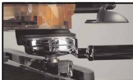
b) Pull the feeder handle (14) towards you to obtain a single measure. Release the handle for it to return to its position.
