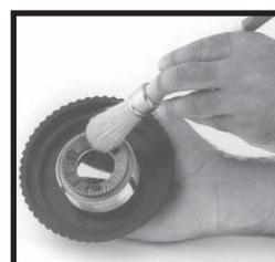
c) Press the adjustment trigger (6) and keep it pressed to free the adjustment platen (4) and turn the platen TOWARDS THE LEFT, in the direction of the "G" arrow, until you remove the platen.
